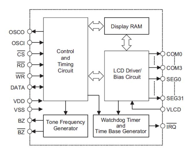
Note:  $\overline{\text{CS}}$ : Chip selection BZ,  $\overline{\text{BZ}}$ : Tone outputs  $\overline{\text{WR}}$ ,  $\overline{\text{RD}}$ , DATA: Serial interface COM0~COM3, SEG0~SEG31: LCD outputs IRQ: Time base or WDT overflow output
