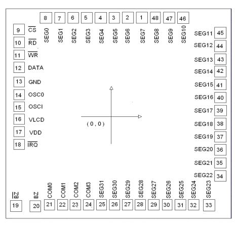
Chip area(with slot): <u>1.614\*1.57</u> um<sup>2</sup> Chip substrate: <u>VDD</u>
